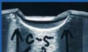
Severe double seam dent plate fracture
