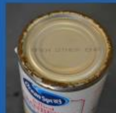
Excessive rusted end
