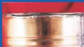
False seam with loss of hermetic seal
