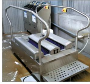
One of the best ways to consistently remove debris and pathogens from all employee footwear is to remove the variability of human behavior from the footwear hygiene process entirely. An <u>automated footwear hygiene station</u> uses mechanized brushes to remove debris while also applying the proper amount of sanitizing solution on footwear to reduce the risk of pathogen spread.
